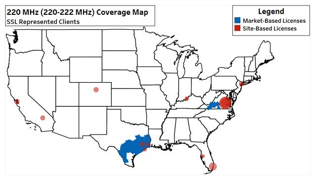
**220-222** MHz spectrum has excellent propagation and can be used for a broad range of applications including fixed & mobile data, voice, and video. Licenses are held and in use for passenger & freight rail communications for rail safety and positive train control (PTC) applications, including I-ETMS (25 kHz of bandwidth, attainable via aggregation of five contiguous 5 kHz channels) and ACSES (12.5 kHz of bandwidth, attainable via aggregation of three contiguous 5 kHz channels).
