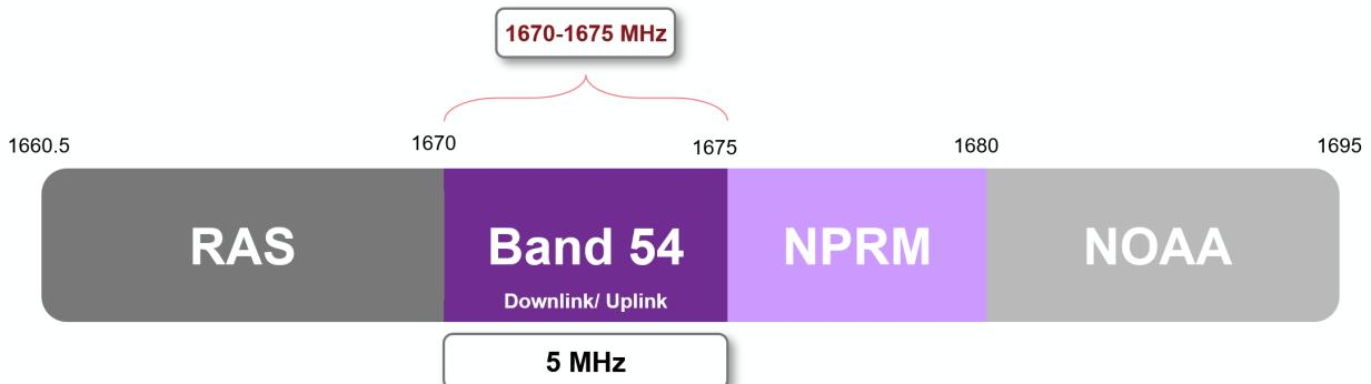
Governed by Part 27 “cellular” rules, Band 54 spectrum has authorized power of 2000 Watts EIRP for base stations and fixed devices, providing unparalleled flexibility and performance for fixed deployments. Consistent with typical vehicular radios, the band has an authorized power limit of 4 Watts EIRP for mobile devices.
