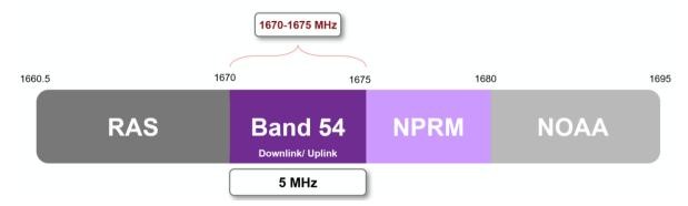
Governed by Part 27 "cellular" rules, Band 54 spectrum has authorized power of 2000 Watts EIRP peak power for base stations and fixed devices, providing unparalleled flexibility and performance for fixed deployments. Consistent with typical vehicular radios, the band has an authorized power limit of 4 Watts EIRP peak power for mobile devices.
