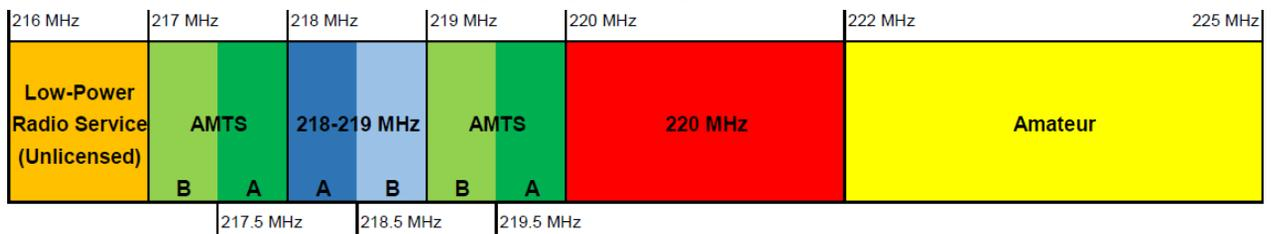
The 220 MHz Band is composed of 5 kHz wide, paired, channel frequencies, with each channel offering a total of 10 kHz capacity. FCC regulations permit aggregation of adjacent channels so that operators may utilize 10 or 15+ kHz wide channels that can support a wide variety of voice and data applications. Please inquire for details on the availability of adjacent channel opportunities.
